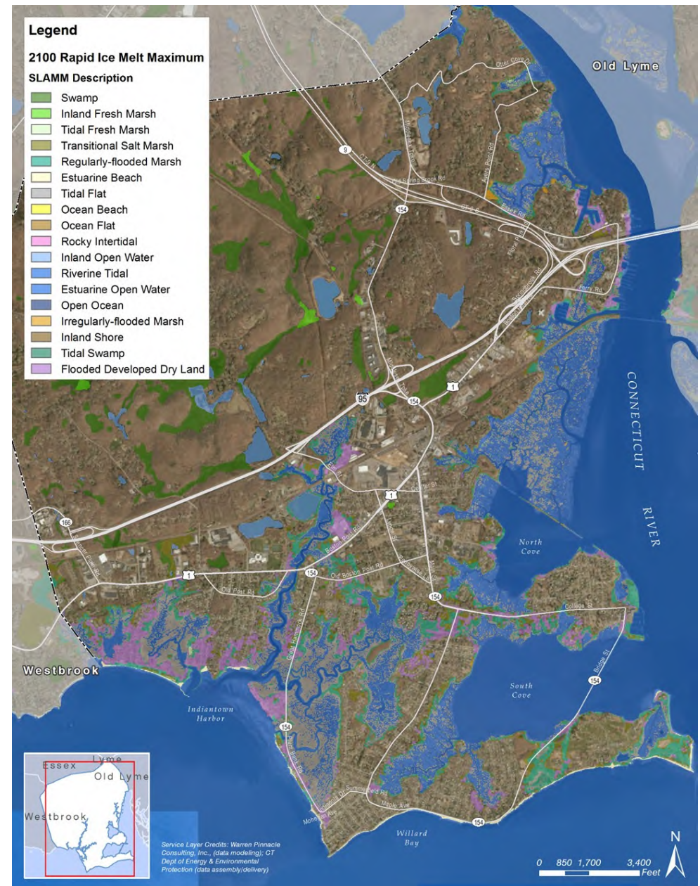
Figure 3-14: SLAMM Rapid Ice Melt maximum simulation of marsh response at Old Saybrook.
