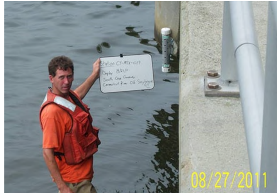
Figure 2-14: Temporary USGS Tide Gage on South Cove Causeway, measuring water levels during Hurricanes Irene and Sandy
